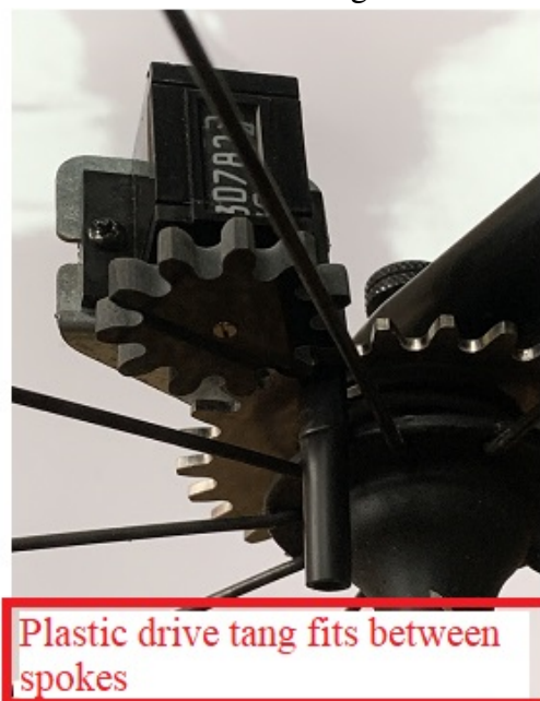
Figure 16: Properly installed counter showing drive tang with plastic extension.
