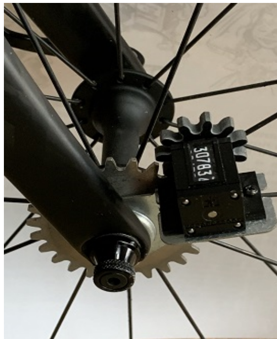
Figure 14. Jones Counter mounted on the front wheel of a bicycle.
