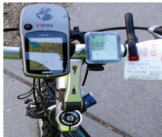
Justin’s bike set up: Jones/Oerth/Lacroix Counter mounted on the headset, Garmin eTrex Vista GPS device, protégé 9.0, and measurement note clip.
