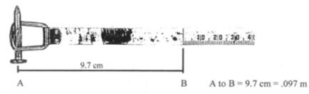
In the above example the zero mark is offset from the pull ring. The distance to the center of the nail is 9.7 cm. This amount should be added to distances which are read on the tape.
