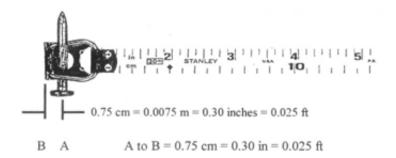
In the above example the zero mark is at the very end of the pull ring. The distance to the center of the nail is 0.75 cm or 0.30 inches. This amount should be subtracted from distances which are read on the tape.
