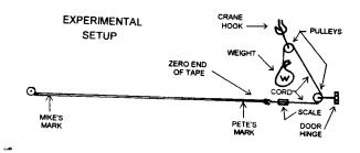
cord, and the cord led through two pulleys, one for horizontal guidance and the second located on a crane hook, so that the sandbag had room to rise. Mike pulled each tape until the sandbag rose from the floor. Pete checked the scale, and recorded the reading at his end of the tape. Mike relaxed, and the second sandbag was loaded onto the cord, and the process repeated.
