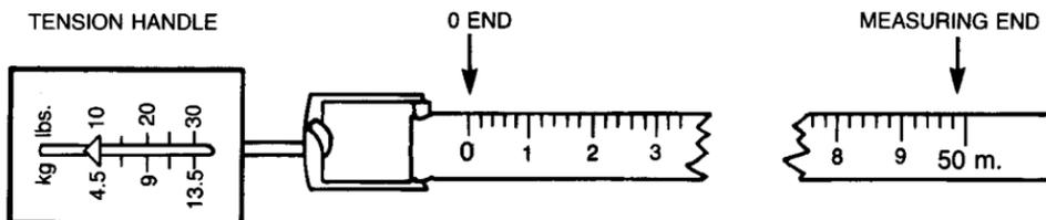
vi) At the end of the kilometer, put your safety glasses on and put a nail in the measuring surface. Put the nail so it is accessible to the bicycle wheel. Measure at a distance from the curb so the cyclists can ride where the kilometer was measured. Paint a circle around the nail. Measure from the nail to curb, and at least two (preferably three) acceptable landmarks (such as manhole covers, fire hydrants, lamppost, corner of building) and take note with a good drawing.
