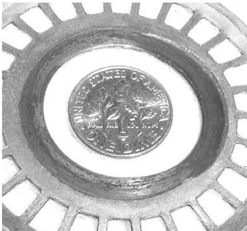
The drive gear after disassembly. Note the eccentric central hole. Measurements show the large diameter to be 2.650 cm, and the smaller diameter 2.535 cm
