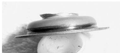
Here we see a side view of the central retainer. Note the groove worn all around the center by the drive gear, almost halfway through the metal. This is certainly one likely cause for sticky and jammed operation.
