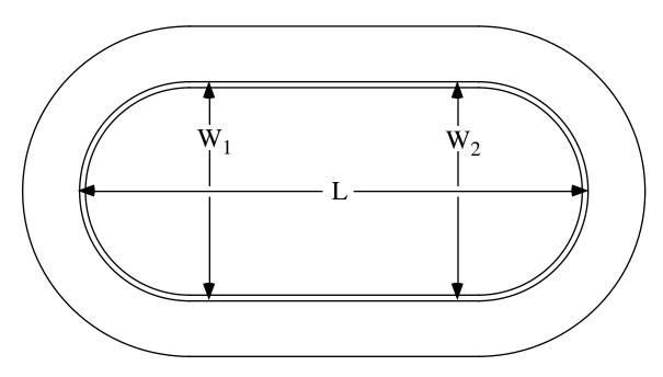
If curb is suitable, then tape circumference directly along outer edge of inner curb. If not, then use "Length-Width" method: Measure distances L,  $W_1$ , and  $W_2$  as shown above, and calculate circumference by the formula:
