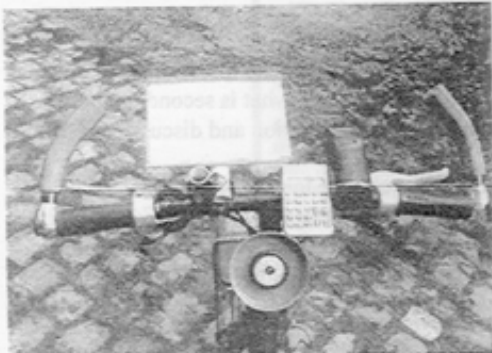
The handlebar display. Calculator and notepad arranged in a convenient way. The round object is a thermometer.
