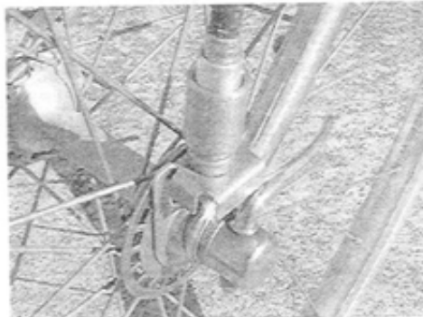
Closeup of speedometer cable attached to Jones counter drive.
