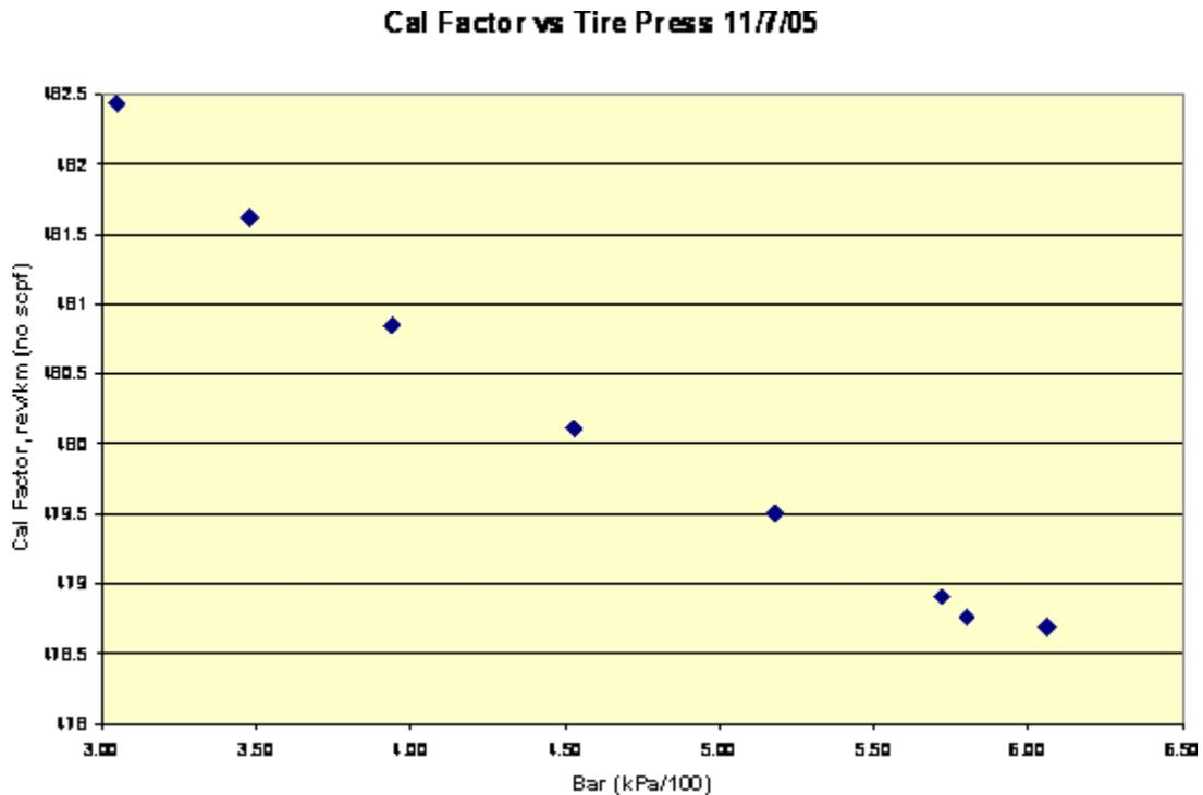
Although a decent straight line may be drawn through all the plotted points, better lines can be drawn through the points below 4 bar, those in the range of 4-5.72 bar, and those at and above 5.72 bar. Moreover the slopes of the lines decrease going to higher pressure. Clearly in going to higher pressures, the pressure coefficient becomes slightly less negative.
