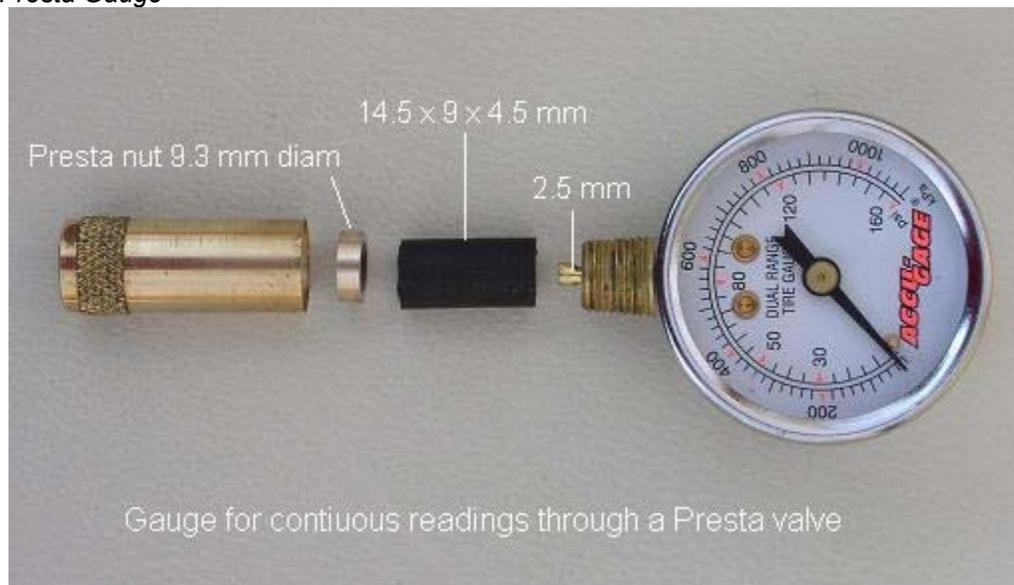
To adjust the diameter of the Presta nut to fit the brass cylinder it was screwed onto the end of the Presta tool to a point at which a burr prevented further rotation. The other end of the tool was fixed into the chuck of a drill which was rotated at high speed over first a coarse file and then a fine one until when the nut was inserted into the large brass cylinder of the gauge, it was a very tight fit. Finally the nut was driven to the bottom of the cylinder.
