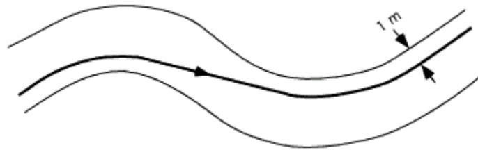
Now, we measure the **shortest possible** route (SPR) that a runner can run. We follow all tangent lines and come to within 0.3 m (i.e., 30 cm or about one foot) of curbs and road edges, as shown in the following diagram:
