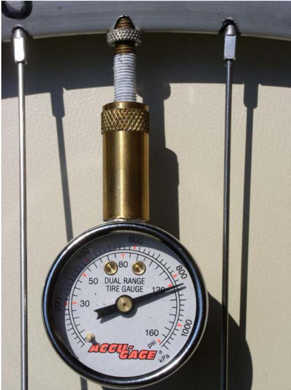
I hope to make a full report soon on my investigations into the pressure-monitoring method for improved efficiency and accuracy in course measurement. However, last Friday I tested a pressure gauge I devised for the continuous monitoring of tire pressure during the certification of "Run for Life" in Raleigh, NC, and results were so good that I feel measurers should learn about it without delay.
